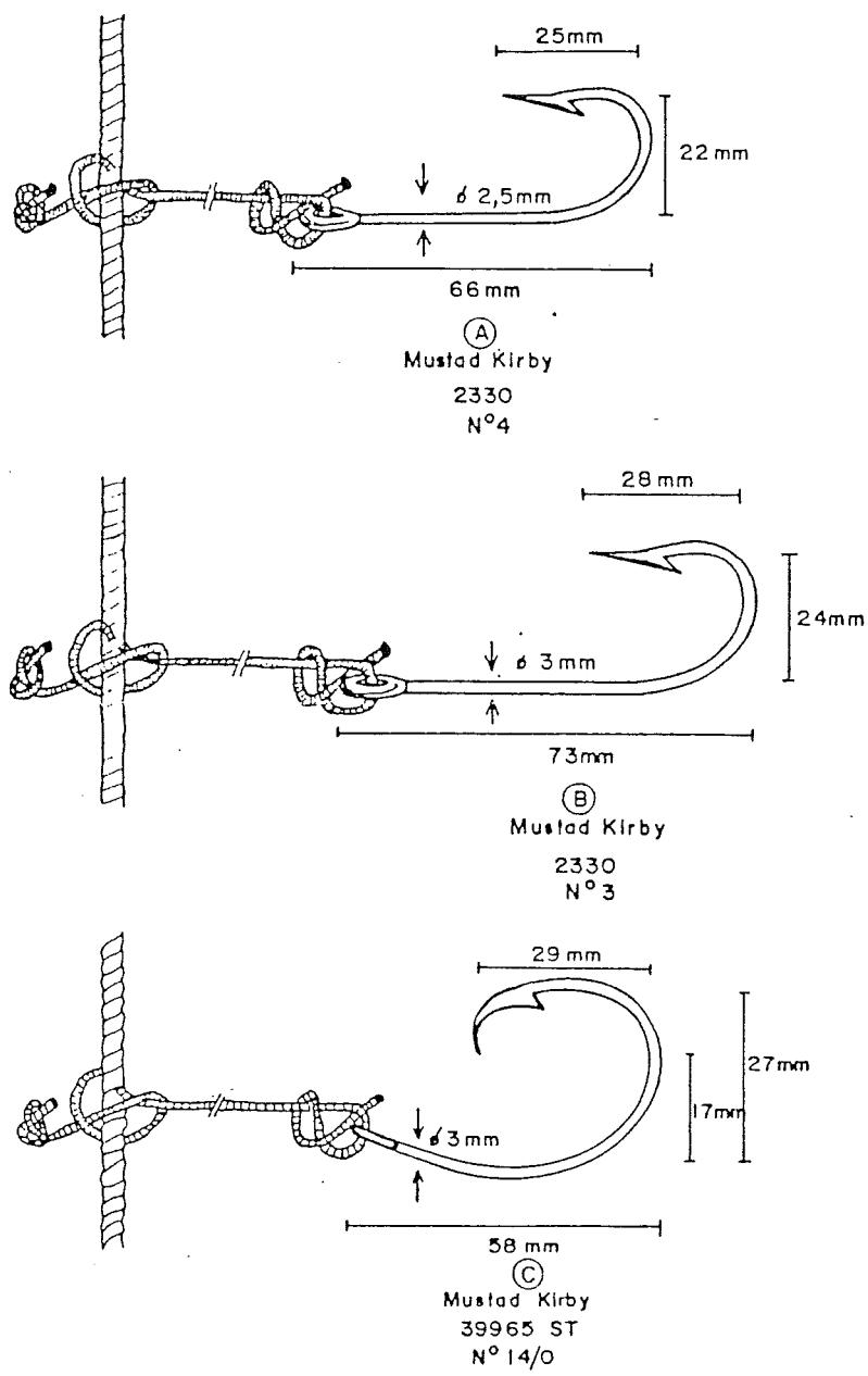
Figure 2: The type of hooks used in the longline fishery of *D. eleginoides* in Chile.
