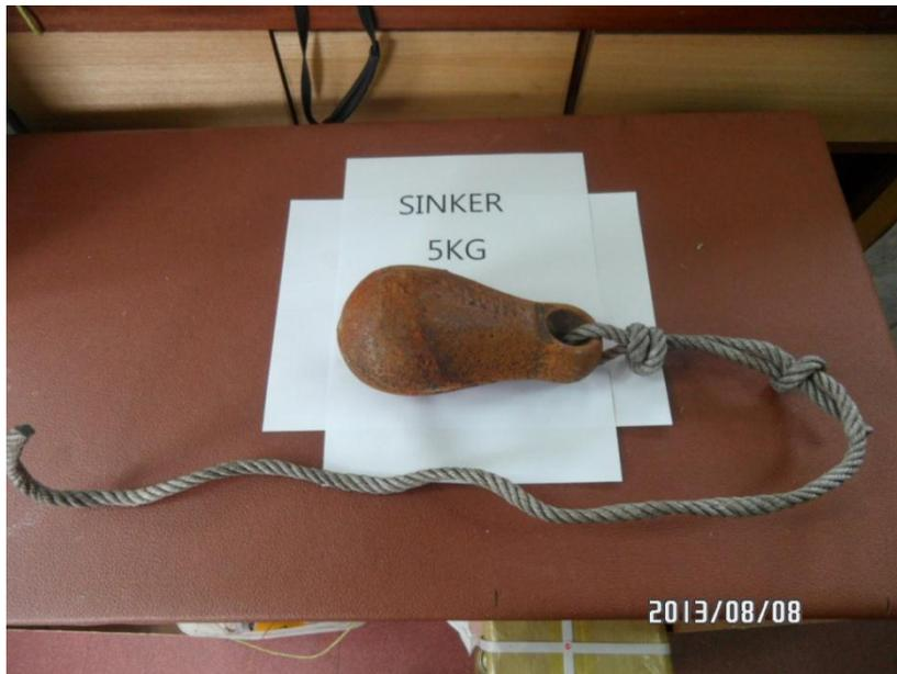
Figure 10 Sinker 5kg
