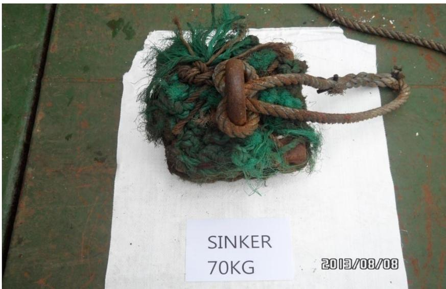
Figure 6. Sinker Weight 70kg
